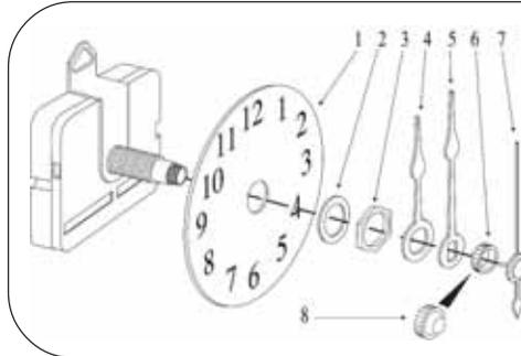
1. Drill a 3/8" hole through the material you are working with and insert the movement.
